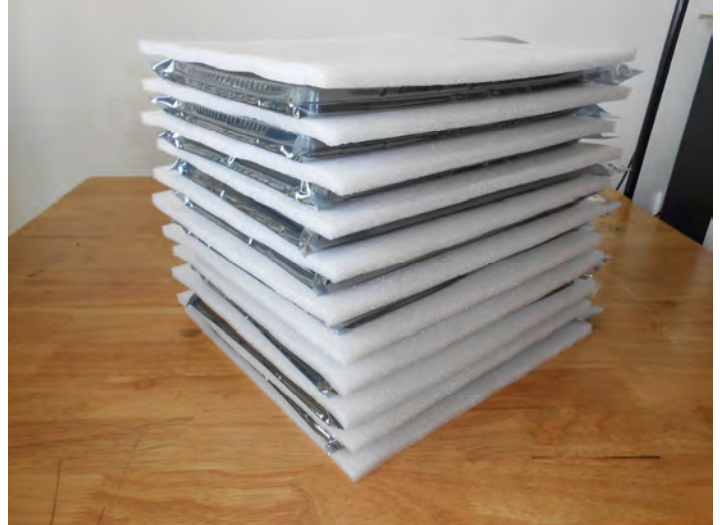
Foam Sheets are Slightly Larger than Trays
